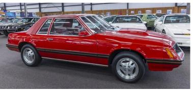
famous. The 2.3 turbo was reported to make 131 hp which was close to 140 hp from the 302, and was available with a four speed in 1979. The Garrett T03 turbo delivered 6 psi of boost. In terms of performance, the 2.3-liter was 70 pounds lighter than the 302 and made almost the same power. The turbo check box also equipped the car with a non-functional hood scoop with "Turbo" badging and a light on the dashboard that glows green under boost and red for overboost.
